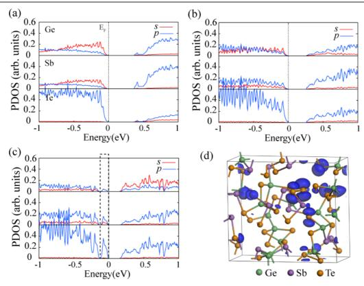
**Figure 3.** The projected density of states (PDOS) for (a) the crystalline phase, (b) the melt-quenched glass and (c) the ideal glass. The Fermi level is set to zero. (d) The isosurface plot of the sum of valence top states in the ideal glass (dashed box in (c)).
