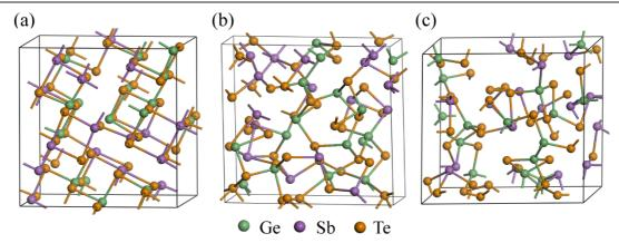
Figure 1. The representative structures of  $Ge_2Sb_2Te_5$  including 72 atoms. (a) The crystalline phase, (b) the melt-quenched glass obtained from a melt-quench process and (c) the ideal glass obtained from a melt-quench simulation on  $Si_2As_2Se_5$ .
