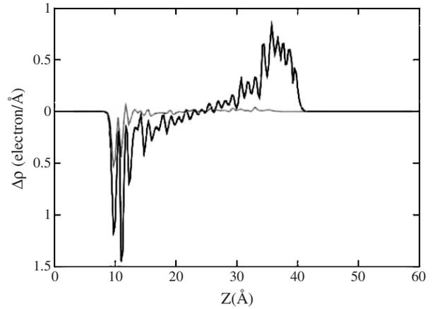
**Figure 2.** The calculated charge redistribution of c-(5, 5)@(10, 10) under an applied electric field of  $0.7 \text{ V } \text{Å}^{-1}$ . The grey and the black curve correspond to the redistributed charge of the inner (5, 5) and outer (10, 10) SWCNT respectively.
