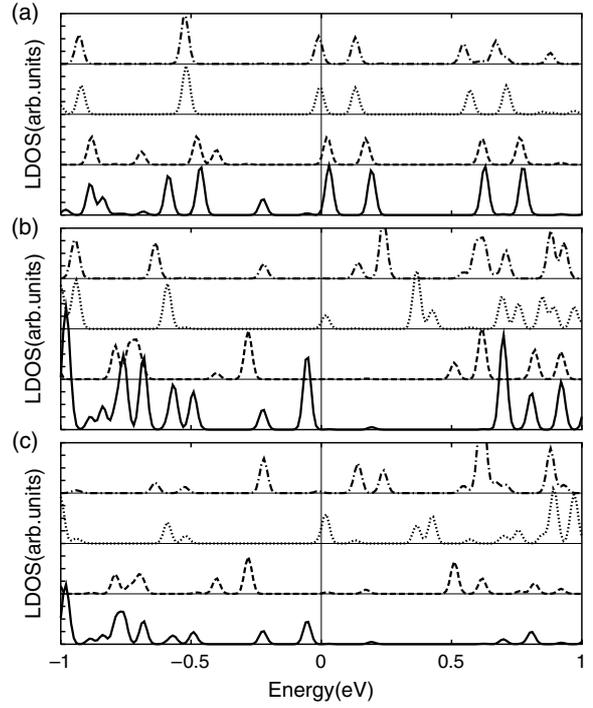
**Figure 4.** The local density of states (LDOS) of b-(4, 4)@(16, 0) at different applied fields projected on (a) the inner (4, 4) nanotube, (b) the outer (16, 0) nanotube, and (c) the bridge atoms. The Fermi level is set to zero in the energy level. The solid, dashed, dotted, and dash-dotted curves represent the LDOS at  $E_{\text{appl}} = 0.0, 0.3, 0.6,$  and  $0.9 \text{ V \AA}^{-1}$ , respectively.
