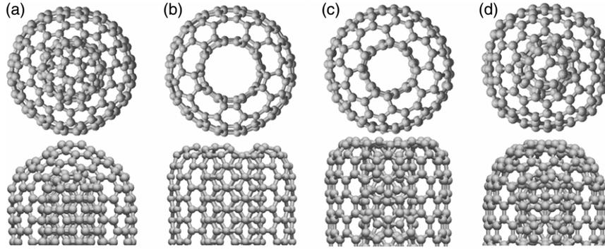
**Figure 1.** The top and the side view of the atomic model of DWCNT tips. The actual lengths in the calculation ( $\sim 30$  Å) are much longer than those appearing in the figure. All dangling bonds of carbon atoms at the bottom are passivated by hydrogen atoms (not shown here). (a) c-(5, 5)@(10, 10) model with the closed domes at the tip. (b) b-(5, 5)@(10, 10) model. The bridge atoms connect edges of each SWCNT. (c) b-(4, 4)@(16, 0) model. (d) c-(4, 4)@(16, 0) model.
